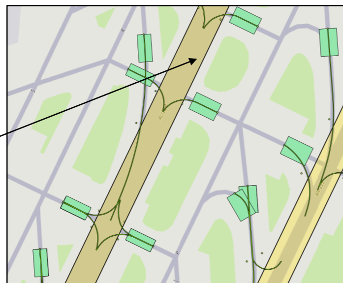
Runway exit polygons at EWR airport
